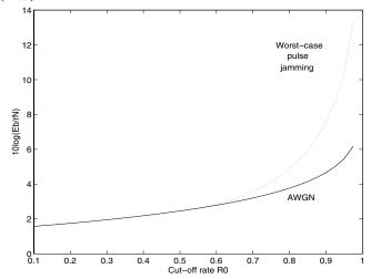
Clearly, there is no penalty in SNR due to worst case pulse jamming for rates below 0.548. Even for  $R_0 = 0.8$  the SNR loss is relatively small. As  $R_0 \rightarrow 1$ , the relative difference between pulse jamming and AWGN becomes large.
