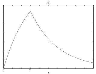
(c)  $y(t) = v(t) \cos 2\pi f_c t$ , where  $f_c >> 1/T$ . Hence the maximum value of y corresponds to the maximum value of v, or  $y_{\text{max}} = y(T) = v_{\text{max}} = v(T) = AT(1 - e^{-1})$ .
