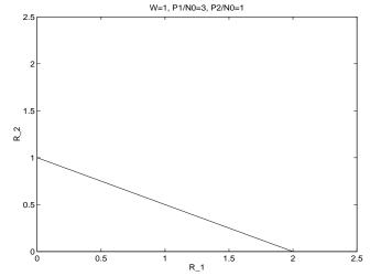
We note that the peak-power-limited TDMA system has a more restricted achievable region  $(R_1, R_2)$ . compared to the FDMA system of problem 15.3.
