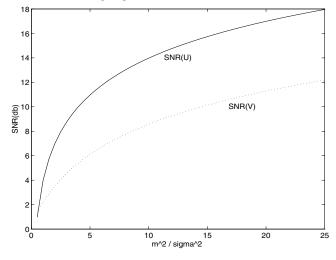
(d) In multichannel operation with coherent detection the decision variable is U as given in (a). With square-law detection, the decision variable is of the form  $\sum_{n=1}^{N} |X_n + jY_n|^2$  where  $X_n$  and  $Y_n$  are Gaussian. We note that V is not the exact model for square-law detection, but, nevertheless, the effect of the non coherent combining loss is evident in the  $(SNR)_V$ .
