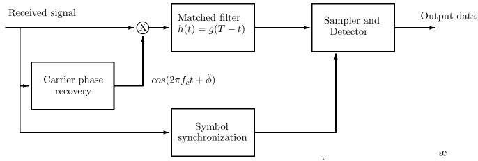
As we note, the received signal is, first, multiplied with  $cos(2\pi f_c t + \hat{\phi})$  and then fed the matched filter. This allows us to have the filter matched to the baseband pulse g(t) and not to the passband signal.
