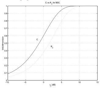
We notice that the difference between the hard-decision cutoff rate and the capacity of the channel is approximately 2.5 to 3 dB.
