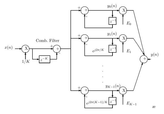
(d) The adjustable parameters in this structure are  $\{E_0, E_1, ..., E_{K-1}\}$ , i.e. the DFT coefficients of the equalizer taps. For more details on this equalizer structure, see the paper by Proakis (IEEE Trans. on Audio and Electroacc., pp 195-200, June 1970).
