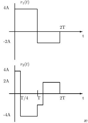
(b) The optimum receiver employs two matched filters  $g_i(t) = r_i(2T-t)$ , and after each matched filter there is a sampler working at a rate of 1/2T. The equivalent lowpass responses  $g_i(t)$  of the two matched filters are given in the following figure :
