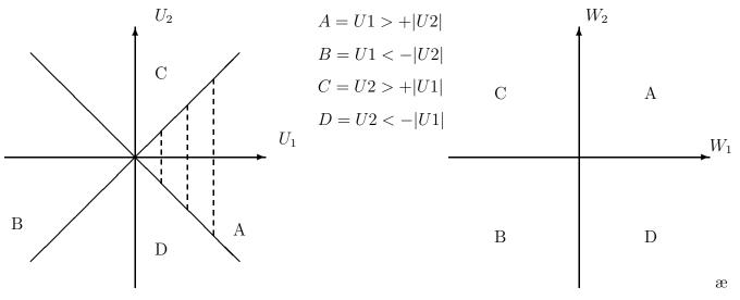
As we see, using the transformation  $W_1 = U_1 + U_2$ ,  $W_2 = U_1 - U_2$  alters the decision regions to :  $(W_1 > 0, W_2 > 0 \rightarrow s_1(t); W_1 > 0, W_2 < 0 \rightarrow s_2(t);$  etc.). Assuming that  $s_1(t)$  was transmitted, the outputs of the matched filters will be :
