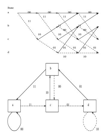
(b) Redrawing the state diagram :
