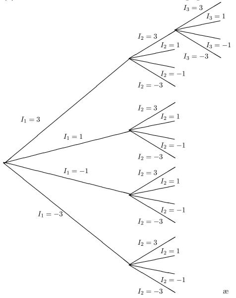
(b) There are four states in the trellis (corresponding to the four possible values of the symbol  $I_{k-1}$ ), and for each one there are four paths starting from it (corresponding to the four possible values of the symbol  $I_k$ ). Hence, 16 probabilities must be computed at each stage of the Viterbi algorithm.
