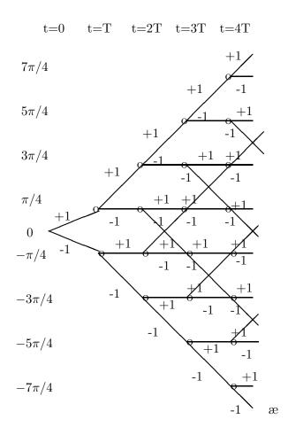
(b) The state trellis is obtained from the phase-tree modulo  $2\pi$ :
