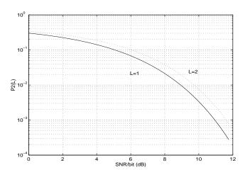
From this graph we note that the combining loss for  $\gamma_b = 10$  is approximately 0.8 dB.
