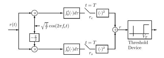
(b) If  $s_0(t)$  is sent, then the received signal is r(t) = n(t) and therefore the sampled outputs  $r_c$ ,  $r_s$  are zero-mean independent Gaussian random variables with variance  $\frac{N_0}{2}$ . Hence, the random variable  $r = \sqrt{r_c^2 + r_s^2}$  is Rayleigh distributed and the PDF is given by :
