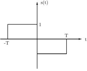
In this case,  $S(f) = T\left(\frac{\sin \pi Tf}{\pi Tf}\right) \sin \pi Tf$ , so that S(n/T) = 0 for all n. Therefore, the condition  $\sum_{k=1}^{K} p_k s_k(t) = 0$  is not necessary.
