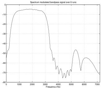
We notice the smoother shape of the PSD, and we can verify that indeed the spectrum is centered around 1800 Hz.
