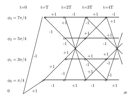
(c) The state diagram is shown in the following figure (with the  $(I_n, I_{n-1})$  or  $(I_{n-1}, I_n)$  that cause the respective transitions shown in parentheses)
