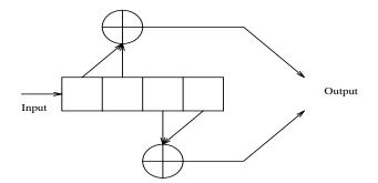
The state diagram for this code has a self-loop in the state 111 with input 1, and output 00. A more subtle example of a catastrophic code is the following :
