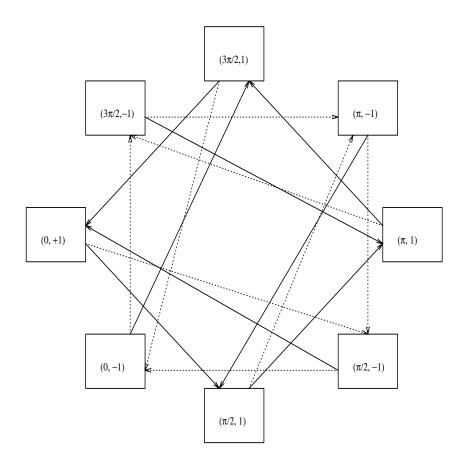
The treatment in Probl. 4.27 involved the terminal phase states only, which were determined to be  $\{\pi/4, 3\pi/4, 5\pi/4, 7\pi/4\}$ . We can easily verify that each two of the combined states, which were obtained in this problem, give one terminal phase state. For example  $(\theta_n, I_{n-1}) = (3\pi/2, -1)$  and  $(\theta_n, I_{n-1}) = (\pi, +1)$ , give the same terminal phase state at t = (n+1)T:
