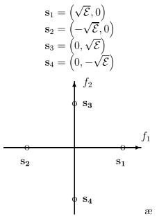
As we see, this signal set is indeed equivalent to a 4-phase PSK signal.
