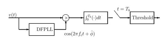
(b) At the receiver (DFPLL) the signal is demodulated by crosscorrelating the received signal :
