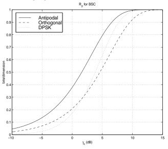
As we see, orthogonal signaling is 3 dB worse than antipodal signaling. Also, DPSK is the worst scheme in very low SNR's, but approaches antipodal signaling performance as the SNR goes up. Both these conclusions agree with the well-known results on the performance of these schemes, as given by their error probabilities given in Chapter 5.
