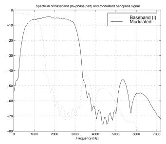
We notice the rather significant sidelobe that is due to the non-completely eliminated image of the spectrum that was generated by the interpolating process. We could mitigate it by choosing an interpolation filter with lower cut-off frequency, but then, we would lose a larger portion of the useful signal as well. The best solution would be to use a longer interpolation filter.
