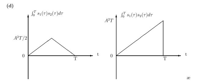
(e) The outputs of the matched filters are different from the outputs of the correlators. The two sets of outputs agree at the sampling time t = T.
