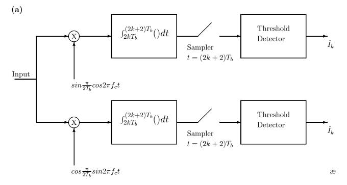
(b) The offset QPSK signal is equivalent to two independent binary PSK systems. Hence for coherent detection, the error probability is :
