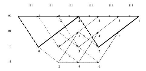
The decoded sequence is  $\{111, 101, 011, 111, 101, 011\}$  which corresponds to the information sequence  $\{x_1, x_2, x_3, x_4\} = \{1, 0, 0, 1\}$  followed by two zeros.
