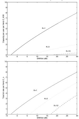
As we observe the normalized capacity per user  $C_K/W$  decreases to 0 as the number of user increases. On the other hand, we saw that the total normalized capacity  $C_n$  is constant, independent of the number of users K. The second graph is explained by the fact that as the
