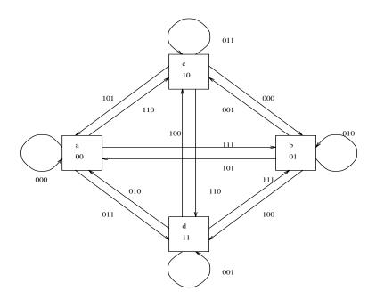
The 2-bit input that forces the transition from one state to another is the 2-bits that characterize the terminal state.
