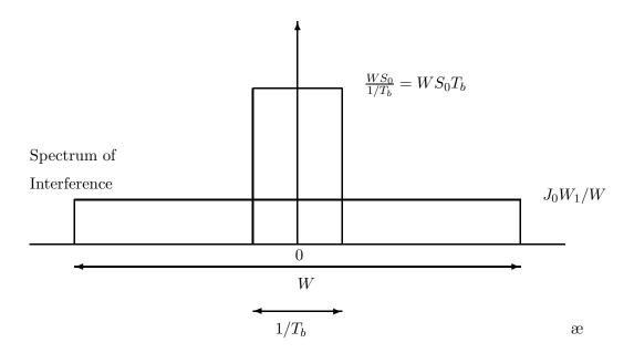
After multiplication with the PN reference, the interference power in the bandwidth  $1/T_b$  occupied by the signal is
