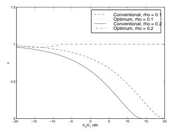
We notice the much better performance of the optimal detector especially when the interfearer (user 2) is much stronger than the signal. We also notice that the performance of the conventional detector decreases as  $|\rho|$  (i.e interference) increases, which agrees with the first observation.
