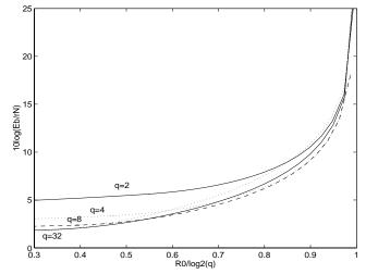
For low rates, the loss due to partial band jamming is negligible if coding is used. Increasing q reduces the SNR/bit at low rates. At very high rates, a large q implies a large SNR loss. For q = 2, there is a 3dB loss relative to binary PSK. As  $q \to \infty$ , the orthogonal FSK approaches -1.6dB as  $R_0 \to 0$ .
